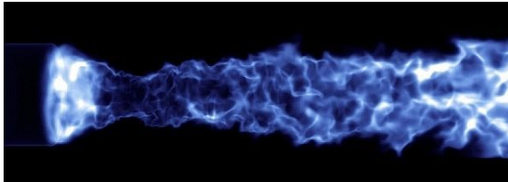
Volume rendering of a non-premixed swirl flame as simulated by LES.
